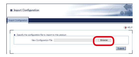
**4.** A window to select the configuration file (**config.txt**) is displayed. Select the file to upload and click **Open**.
