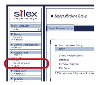
**4.** Enter the PIN code of wireless device at **PIN Code** under **Smart Wireless Setup Execute** and click **Register**.
