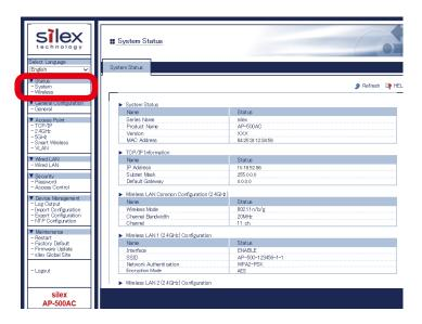
If you click **Wireless**, the status page for wireless station devices is displayed. In this page, you can check the MAC Address, RSSI (wireless signal strength) and IP Address for the connected wireless station devices.
