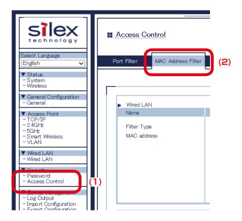
**5.** Select the wireless interface assigned for WDS connection and check that the MAC Address filter is not set to block access from the client AP.
