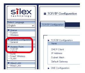
**3.** Select **DISABLE** for **DHCP Client** and configure a static IP Address.
