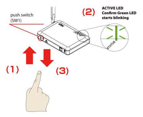
2. Press the wireless setup switch also on your wireless device.
