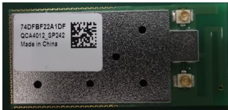
The custom dual-band low-energy, low-power SX-SP242 module Silex Technology Developed for Elemental Path's second-generation CogniToy.
