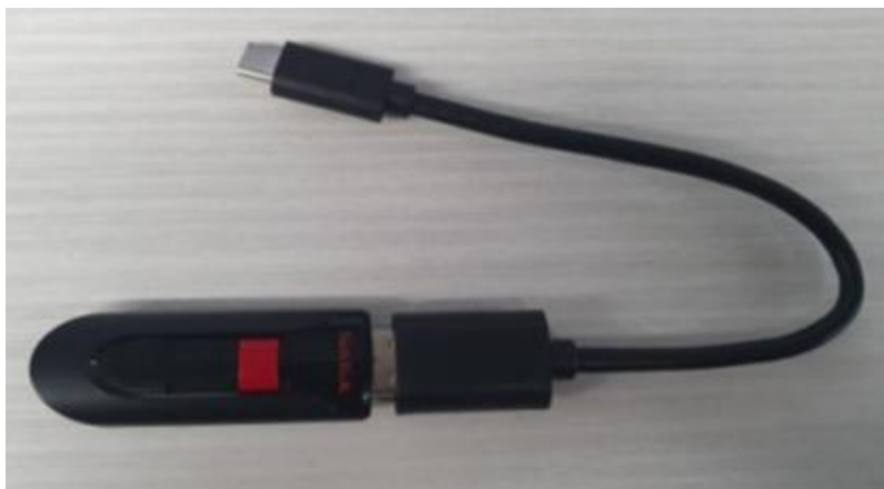
Figure 10 shows USB-C to USB-A adapter connections.
