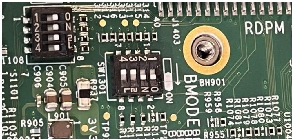
Figure 6. i.MX93 EVK Boot switch
