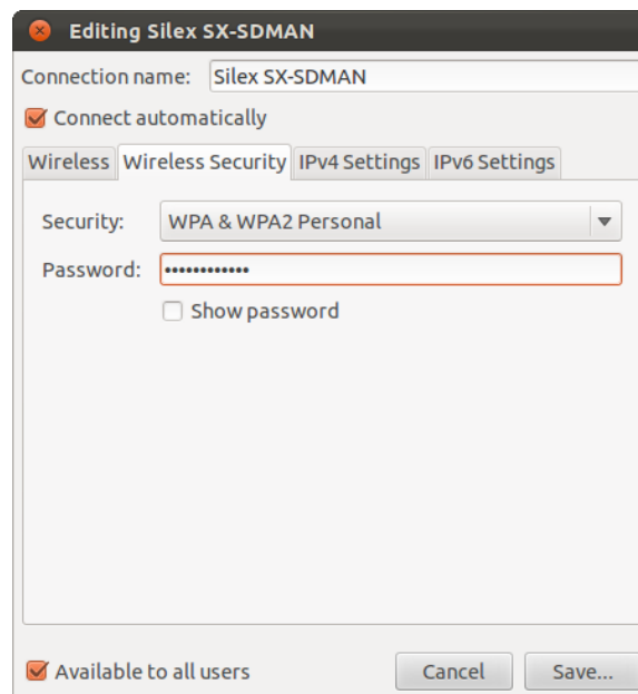
Figure 7 - WLAN Network Configuration WPA/WPA2 Setup
