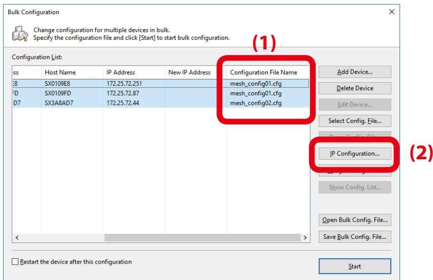
8. Specify the IP address range to configure for BR-400AN units (1).
