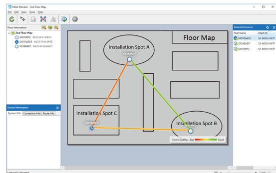
As shown in the image above, the actual installation environment is simulated on Mesh Monitor. The route information is displayed based on the actual route setting of BR-400AN. It is possible to change some functions of BR-400AN using Mesh Monitor (e.g. enabling/disabling Access Point function, etc.). Also, a history of Mesh network route and BR-400AN's operating status can be checked and which can be used conveniently for troubleshooting.
