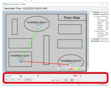
**3.** The information corresponding to the slider position is displayed. By looking at the detailed information of floor map and Mesh device, you can check the network status as of the recorded time.
