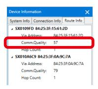
When a Mesh device is selected and the other Mesh device is right-clicked and **Display** Route to This Device is clicked from the context menu, the route from the selected Mesh device is displayed.
