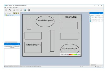
2. Drag and drop a Mesh device on the floor map from the device list.
