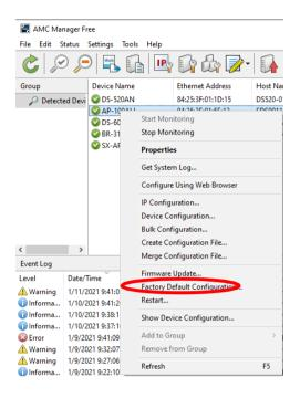
2. Check the check box of Restart the device after the factory default configuration, and click Reset. The pop-up window appears, then click Yes.
