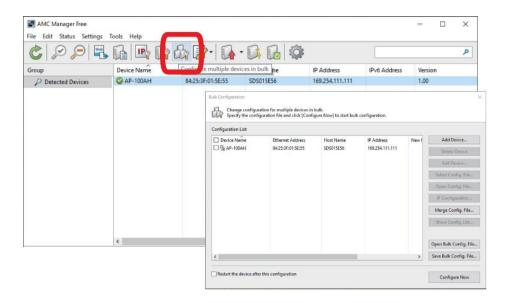
**5.** Select the AP-100AH unit to configure from the **Configuration List** (1) and click the **Select Config. File** button (2) in the **Bulk Configuration** window. When a file selection dialog appears, select the created configuration file and click **Open.**
