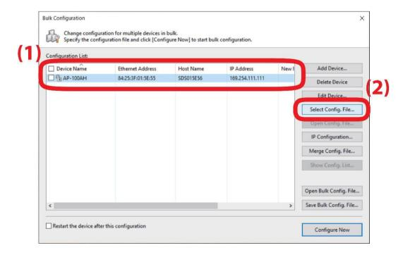
**6.** Check the check box of the AP-100AH unit to configure (1) and click **Configure Now** (2).
