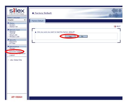
**3.** After the factory default configuration is completed, the AP-100AH will automatically restart. The web configuration page can be accessible again through the Ethernet port by 169.254.111.111.
