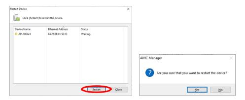
**3.** Enter the password for the AP-100AH and click **OK.** When the restart finishes, **Status** changes to **Completed.** (Password window appears only when the password is set.)
