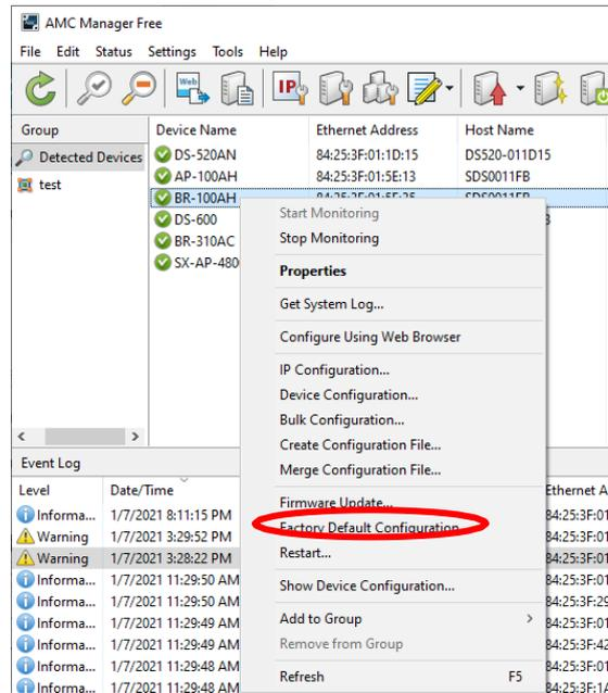
2. Check the check box of **Restart the device after the factory default configuration**, and click **Reset**. The pop-up window appears, then click **Yes**.
