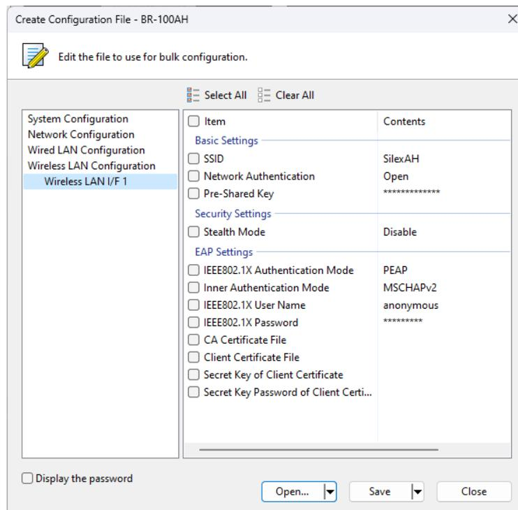
4. Select the BR-100AH unit to configure from the device list of AMC Manager®, and click the icon **Configure multiple devices in bulk**.
