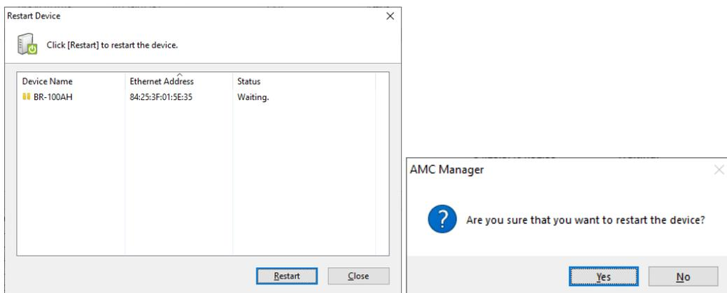
3. Enter the password for the BR-100AH and click **OK**. When the restart finishes, **Status** changes to **Completed**. (Password window appears only when the password is set.)
