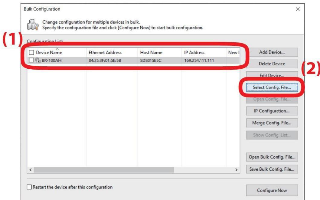
6. Check the check box of the BR-100AH unit to configure (1) and click **Configure Now** (2).
