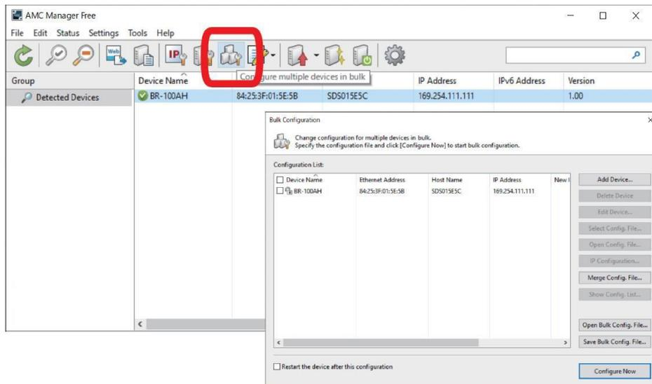
5. Select the BR-100AH unit to configure from the **Configuration List** (1) and click the **Select Config. File** button (2) in the **Bulk Configuration** window. When a file selection dialog appears, select the created configuration file and click **Open**.
