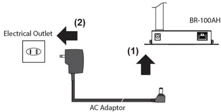
**3.** Turn on the non-wireless device connected to the BR-100AH. When the wireless network is established, all LEDs turn on. The BR-100AH will be ready to use. You can use the non-wireless device over a wireless network.
