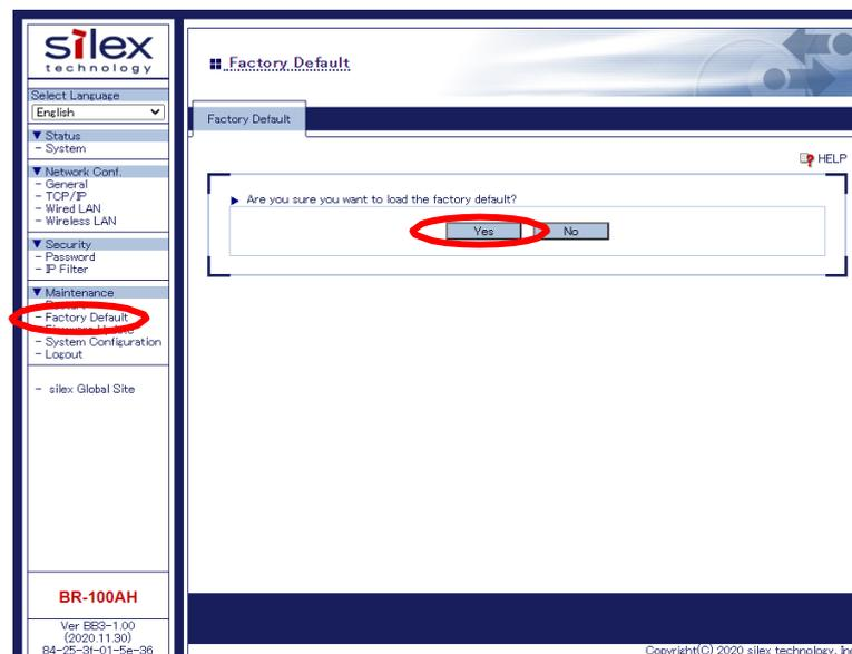
3. After the factory default configuration is completed, the BR-100AH will automatically restart. The web configuration page can be accessible again through the Ethernet port by 169.254.111.111.
