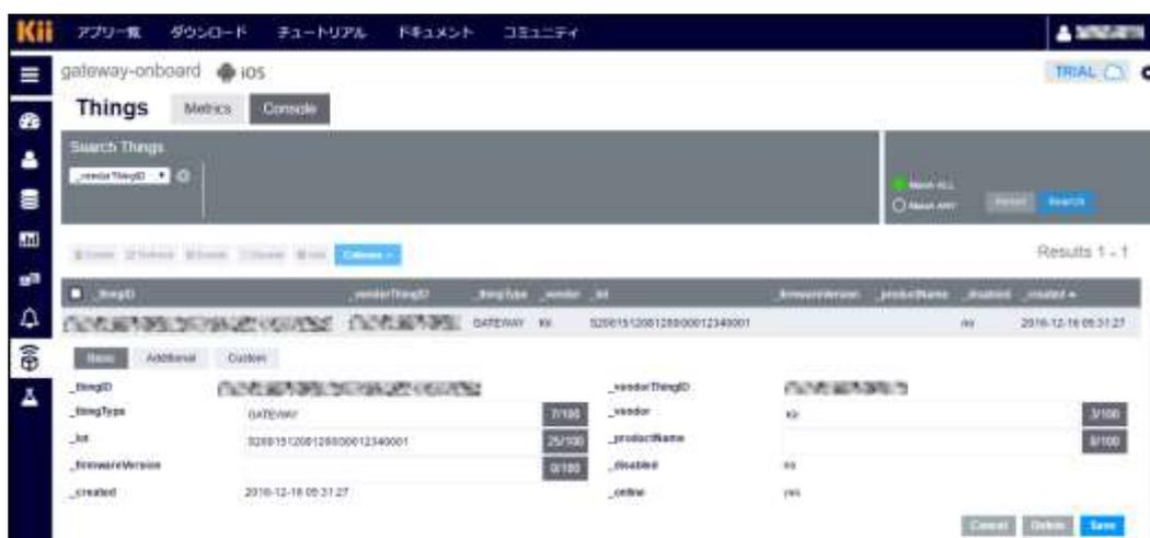
When LB-100AN operates properly, it uploads the temperature information from the converter periodically (initial setting: 10-second interval).
