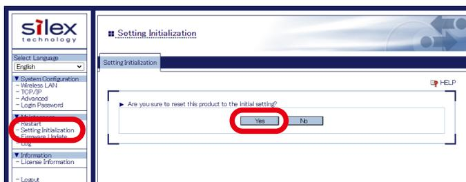
3. After the factory default configuration is completed, the BR-500AC will automatically restart. When the POWER LED turns green after all LEDs turn off, the restart is completed.
