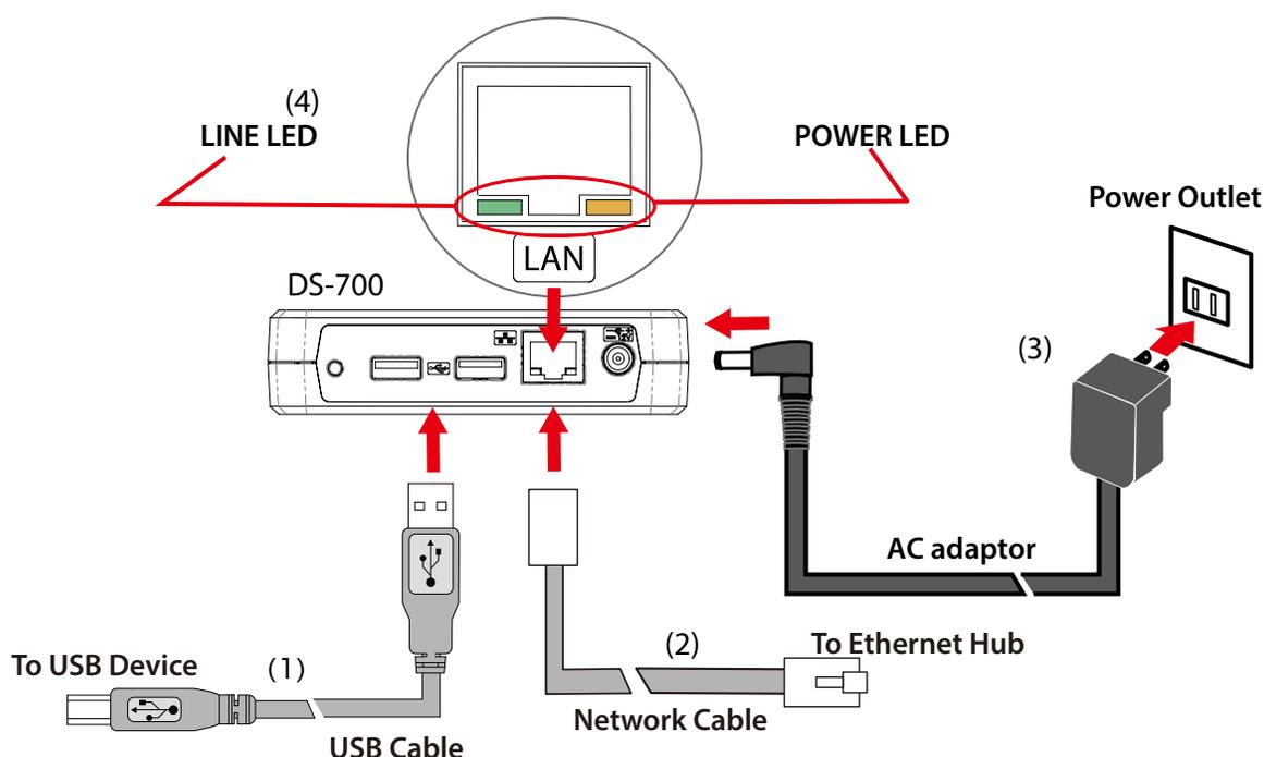
1. Connect DS-700 and the USB device using a USB cable (1).
