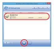
Once you successfully link to the serial device, the status icon is changed to "Connected" in the SX Virtual Link for Serial Device Server's main window.
