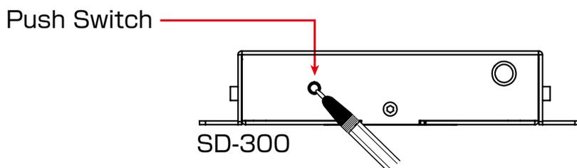
2. The factory default configuration will begin when the push switch is released.
