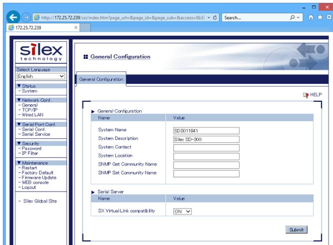
The screenshot shows the Silex SD-300 web interface. The left sidebar contains a navigation menu with categories like Status, Network Conf., Serial Port Conf., Security, and Maintenance. The main content area is titled 'General Configuration' and contains two sections: 'General Configuration' and 'Serial Server'. The 'Serial Server' section has a table with the following data:
