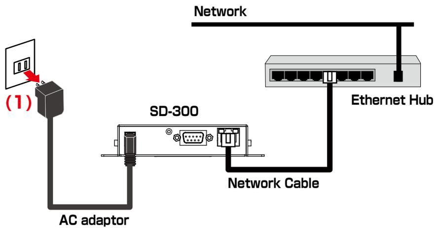
11. Connect the serial device that you wish to share over the network to SD-300 using a serial cable and insert the power plug of SD-300 into the outlet.
