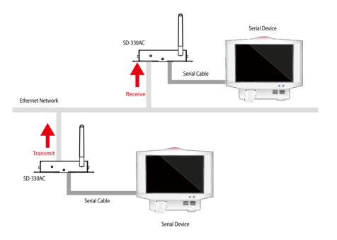
When SD-330AC's are communicating with each other using Ecable Mode, the transmitter end sends the serial port data to the receiver end, and the receiver end sends it to the serial device.
