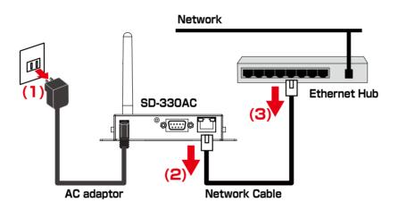
**6.** Connect the serial device that you wish to share over the network to SD-330AC using a serial cable and insert the power plug of SD-330AC into the outlet.
