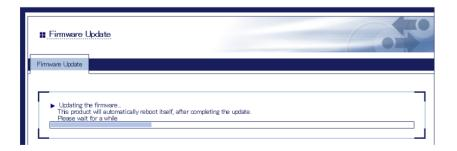
**6.** When the system status page is displayed, the firmware update is completed. See the bottom left of the page and check that the version information is changed.
