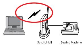
Establish PC to StitchLink II wireless connection via Wireless Access Point/Router (Infrastructure mode).
