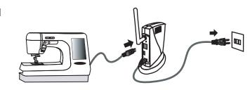
Connect the sewing machine to be shared over the network along with this product via a USB cable, and insert the power plug into the outlet.
