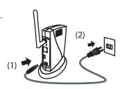
ii. Connect the power supply to this product, and then insert the AC Plug into the electric outlet.
