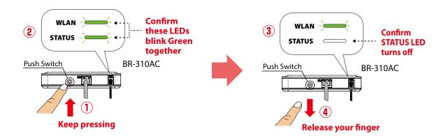
**6.** The BR-310AC and the Access Point will start to communicate each other. When the configuration finished successfully, the WLAN LED turns Green and the STATUS LED turns or blinks Green.
