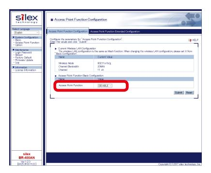
**4.** The detailed setting of Access Point feature such as SSID, authentication method, etc. can be configured. For details on the configurable items, refer to **5-1. Configuration Items on BR-400AN's Web Page** - **Access Point Function Configuration Page**. The wireless mode, channel bandwidth and channel cannot be changed in this page. To change these settings, go to the **Basic Configuration** page.
