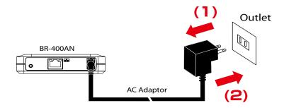
**2.** When the POWER LED turns green and WLAN LED turns or blinks green/orange, the restart is completed. After the restart, the BR-400AN will start in a normal mode.
