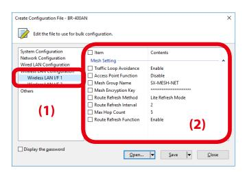
**4.** Select **Enable** for **Access Point Function** and check the check box.
