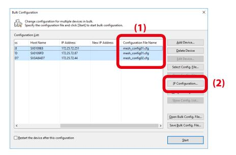
**9.** Specify the IP address range to configure for BR-400AN units (1). When the setting is finished, click **OK** (2).
