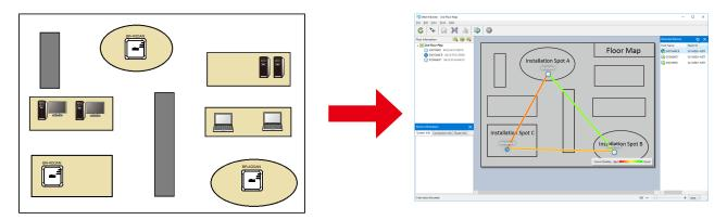
As shown in the image above, the actual installation environment is simulated on Mesh Monitor. The route information is displayed based on the actual route setting of BR-400AN. It is possible to change some functions of BR-400AN using Mesh Monitor (e.g. enabling/disabling Access Point function, etc.). Also, a history of Mesh network route and BR-400AN's operating status can be checked and which can be used conveniently for troubleshooting.
