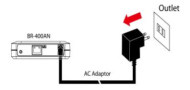
2. Press and hold the push switch on the front (1) while inserting the AC adaptor back into the electrical outlet (2).
