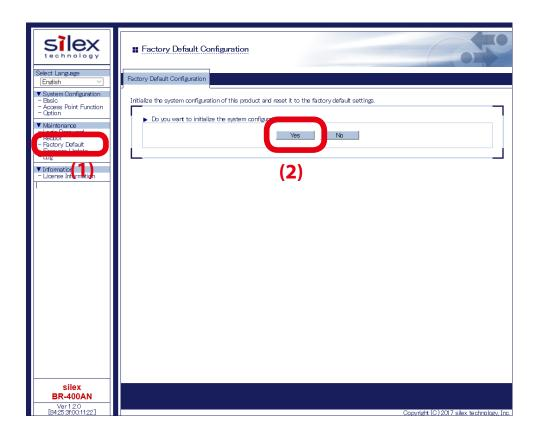
**3.** When the factory default configuration is completed, BR-400AN is automatically restarted. When the restart is completed, the POWER LED turns green and the WLAN LED turns or blinks green/orange. BR-400AN will run in a normal mode then.
