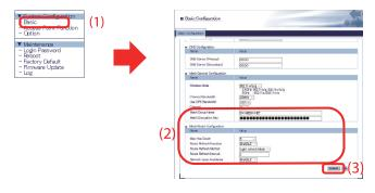
\* The wireless setting (Wireless Mode, Channel Bandwidth, Channel) or Mesh Group Name and Mesh Encryption Key must be the same for all devices on the Mesh network.
