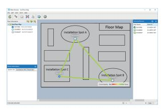
It is also possible to configure a part of BR-400AN's functions on Mesh Monitor (e.g. enabling/disabling Access Point function).
