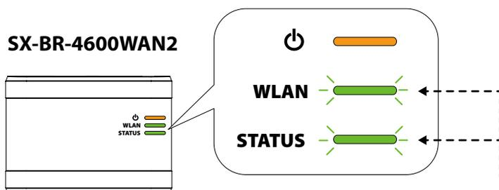
**The LEDs flash alternately during the MAC address resolution**
