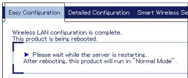
When you wish to bridge the PC used for this configuration wirelessly, restart the PC. To bridge another device wirelessly, turn off both SX-BR-4600WAN2 and PC, remove the SX-BR-4600WAN2 from the PC and connect the SX-BR-4600WAN2 to the device you wish to use wirelessly using a network cable. For details, refer to **Connecting Non-wireless Devices** in the next page.
