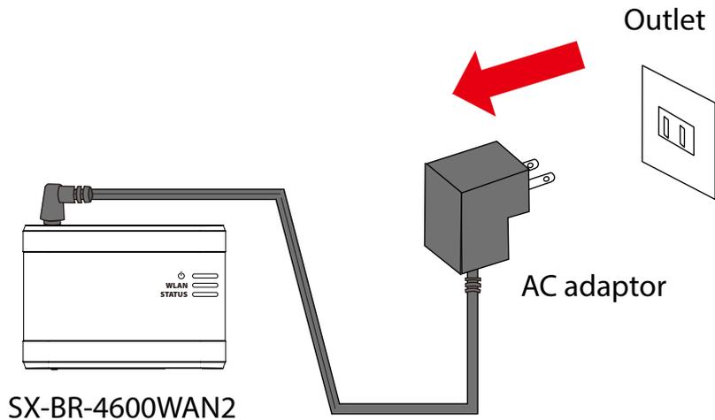
2. Press and hold the push switch on the front while inserting the AC adaptor back into the electrical outlet.
