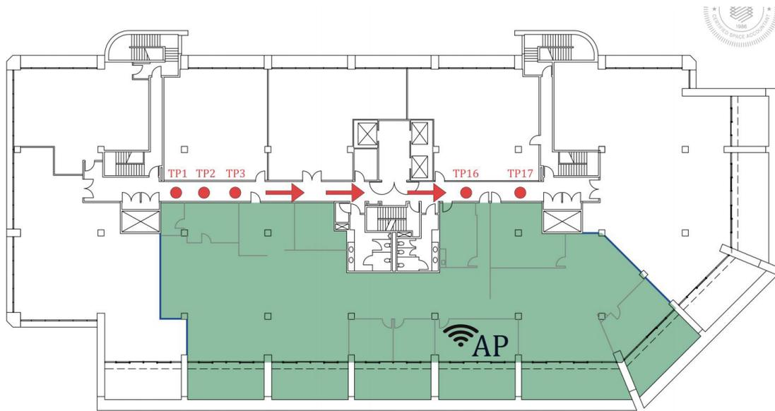
*Figure 1: Second floor of the Sillex office building; red arrows demonstrate the location of test points, and AP abbreviation identifies each access point location.*
