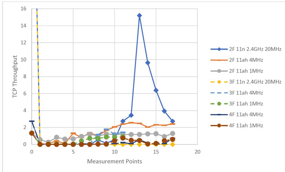
Figure 2: Data throughput at different test points on floor two
