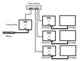
If you plan to use the X-5 on a wired network, configuration is not necessary. You can use the X-5 with the default settings.
